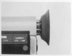
the eyepiece can be rotated freely. Next turn the eyepiece until both a distant image and the edges of the frame appear clearest to you. Then lock the eyepiece in this position by turning the eyepiece lock as far as it will go in the direction of the arrow. Once the eyepiece is adjusted, there should be no reason to change it unless the cameraman or his eyesight changes.
