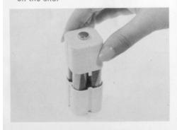
Reinsert the plastic case into the battery chamber, align the dots on handgrip body and cap, push cap on, and secure it by turning lock to C position.
