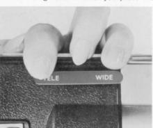
TELE side of the power zoom control or use the manual zoom lever to increase the focal length, your subject image becomes larger; pressing the WIDE side or decreasing the focal length makes it smaller. Power or manual zooming can be used for adjusting focal-length to subject distance for composing or cropping before filming or for useful or impressive effects during filming.
