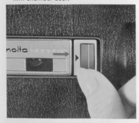
2. Slide the cartridge into the camera from the rear and angled slightly down toward camera front as shown, with the center hole down, the label up, and the opening with film visible toward the front. Then push down gently on the rear edges of the cartridge until it seats flat in the chamber and you hear a click.
