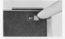
Inserting and removing film cartridges
