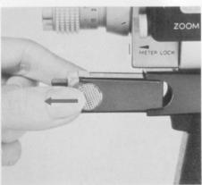
By grasping the knurled round grips on either side of the filming button with thumb and forefinger, the regular filming switch assembly is easily detached from the camera. Electrical connections of the release cord, Intervalometer-P or -S, wireless remotecontrol unit, or tape recorder-control cord can be inserted in its place in the socket.
