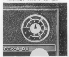
3. Turn the camera to a bright direction and move your hand back and forth in front of the lens to confirm that the F-number scale is working. If it does not move with adequate light, make sure the meter lock button is pushed in to its unlocked position. (If the viewfinder appears completely black, remove the lens cap and/or open the viewfinder shutter.)
