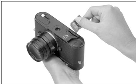
2. Remove the bottom cover (1.36) of the camera.
