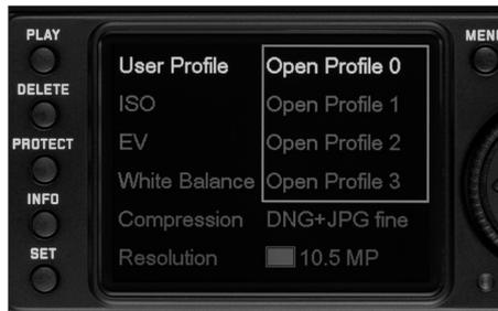
3. To set the respective function, first press the **SET** button (in the picture parameters menu, press it again).
